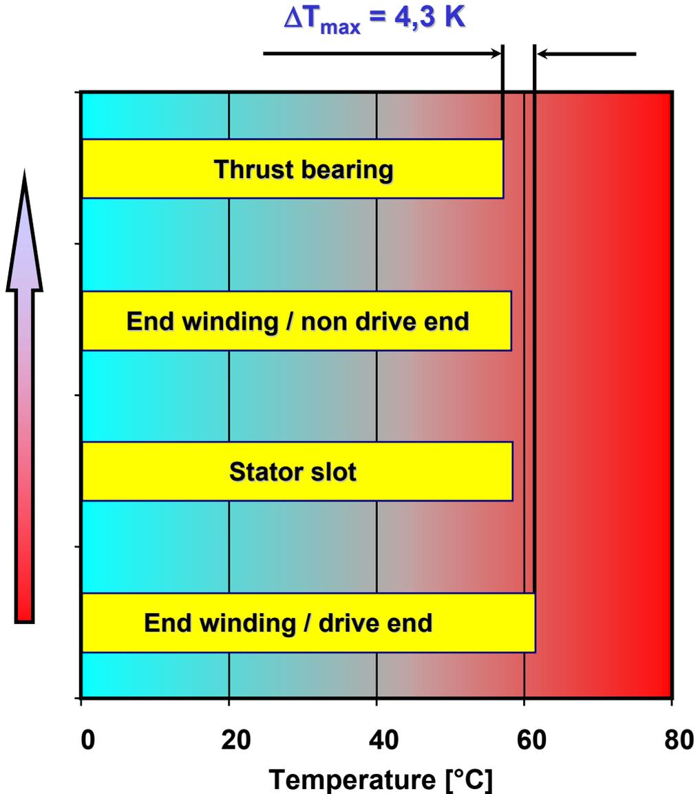
**Small temperature differences due to effective cooling circuit**
